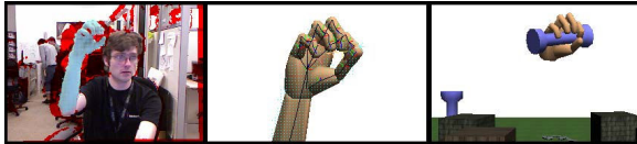
Figure 14: Interacting with a barbell where geometry and collision (instead of gestures and custom programming) enables the grasping, holding, and manipulating of the object.
