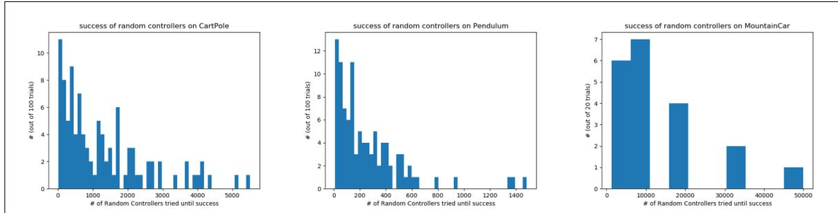
Figure 2. Histograms demonstrating the performance of Uniform Random Search on solving three different problems (left-to-right): controlling an inverted pendulum, performing a swing-up and control of an inverted pendulum, and a MountainCar task. More details are in section 3.1. Success in this case is defined as having a trial which solves the problem within the OpenAI timestep limit (200 iterations)
